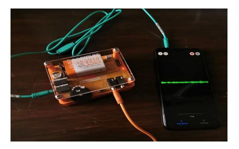
There are 2 labels marked on the Green audio cable. One end is labeled with "SpikerBox" which goes into the SpikerBox and another one is labeled with "Smartphone" which goes into your Android phone, tablet or other mobile devices.
