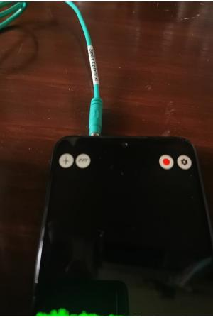
Important thing to mention is that the Green audio cable is only a mono audio input and it doesn't provide stereo or 2 channels.
